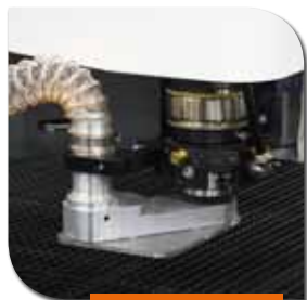
Suction inlet on the cutting head
