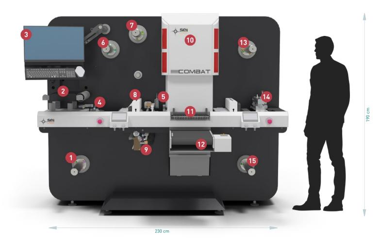
Combat, designed for 360 mm [14,2"] web width, is available in **3 laser configurations** (V150, V300 and V500). It is meant to meet even the most demanding production requirements.
